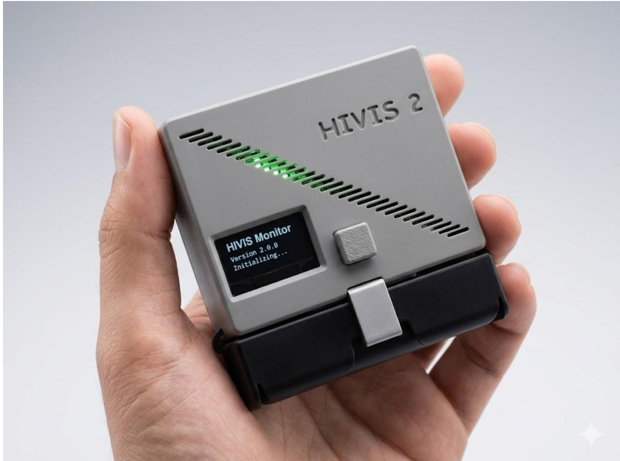
Figure 7 Enclosure with External 18650 Battery
